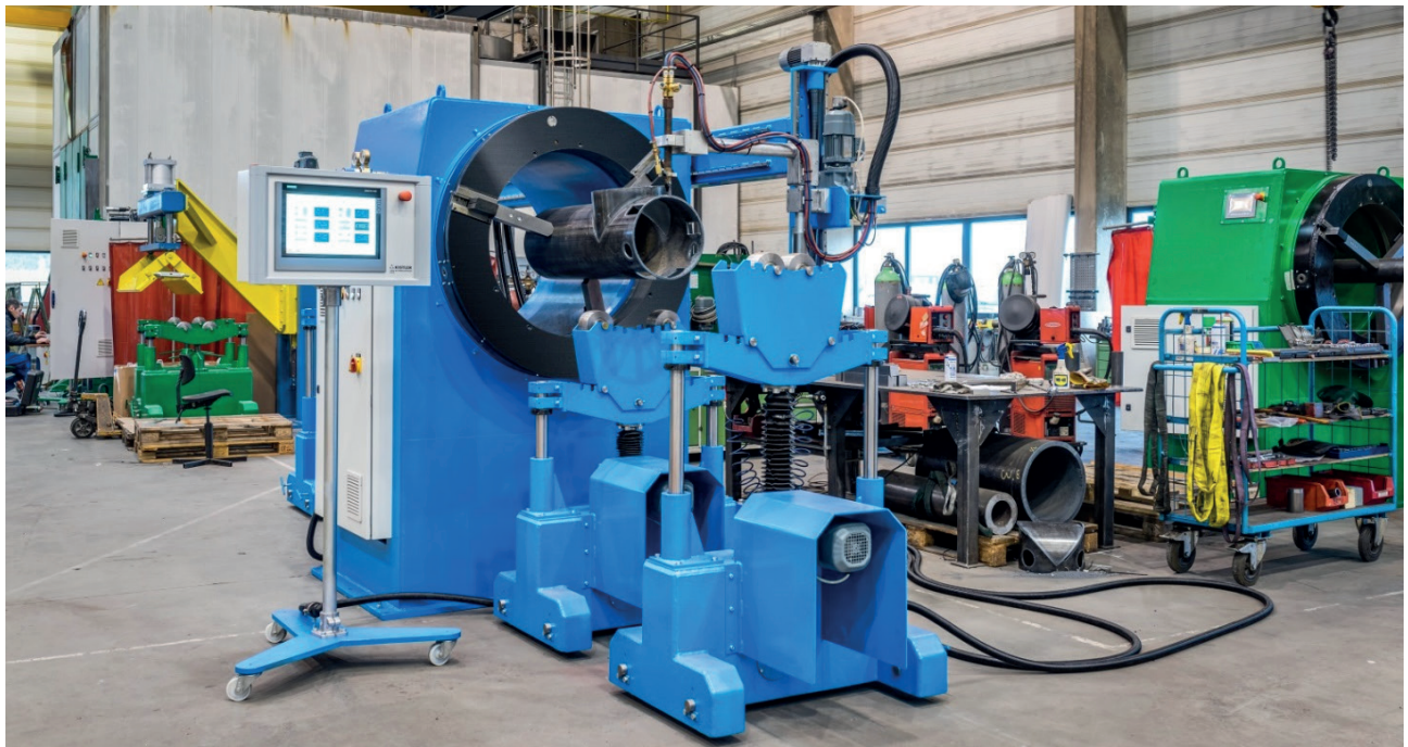
SCM 630 prepared for Plasma Cutting, with 3rd controlled axis (allows bevelling of end cuts) and 540 mm through hole chuck.
