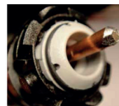
Image 3: A range of possibilities are possible: single wire and tandem wires (Twinarc®)
