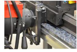
Beveling greater lengths of plate is accomplished with additional sections of guide tracks.
