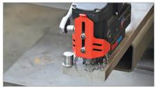
Max milling capacity up to 1-3/8" (36 mm)
