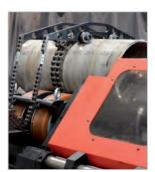
Clamping device for short pipes of 15-3/4" – 32-11/16" length
