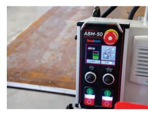
The ABM50 creates bevels with a maximum bevel width of 2" (50 mm) at 45 degrees.
