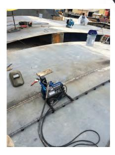
The Arc Runner can be used with the innovative Steelmax flexible guide rail system.
