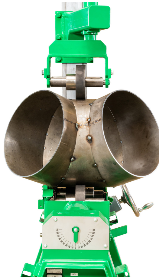
Clamping and rotating of a shallow bend lobster back.
